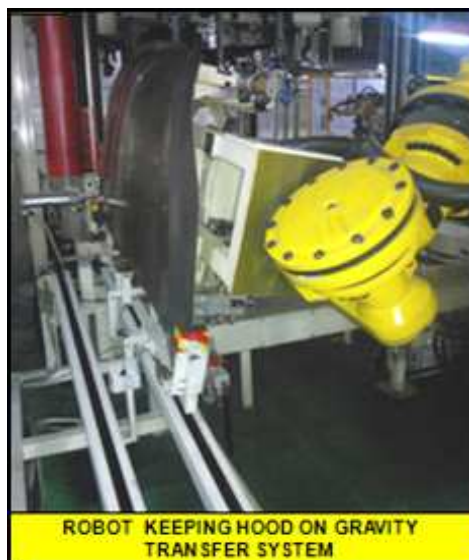
Fig. 4 Gravity transfer system
